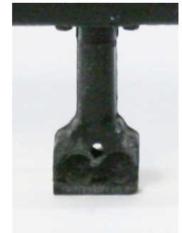
Edges trimmed Holes milled
